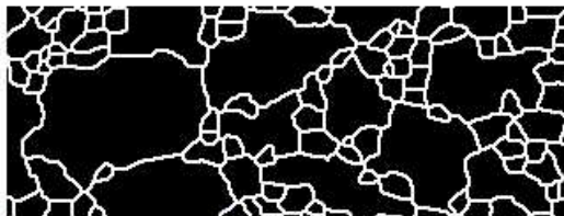
bitmap showing grains in black and grain boundaries in white
